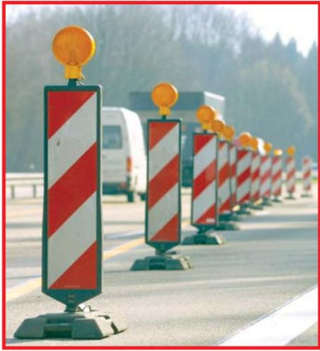
**Guide-light-systems for roadwork sites- AL 12/24 V DC,** complete with a 13 m cable and plug connection, 1 electricity supply cable, 1 connection box with pole-reversal- and low-voltage protection, lamps: diameter 180 / 200 mm, yellow
