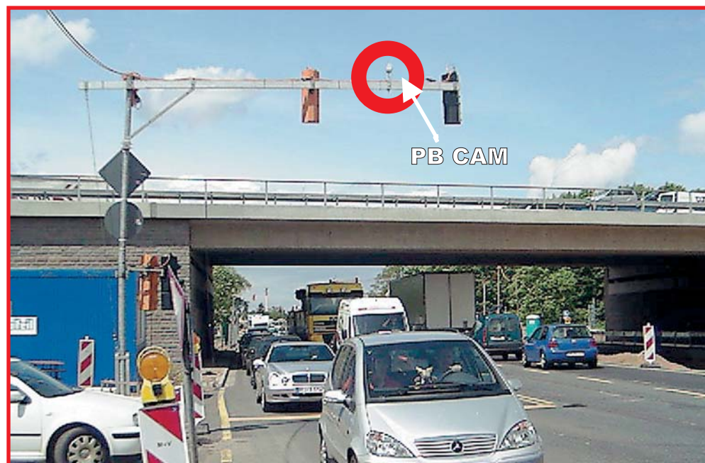
Our camera PB CAM puts aside luxurious attaching of contact loops in the highway cover
