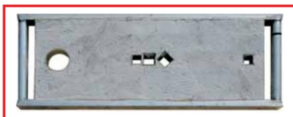
**New foundation plate with a fitting for a 100 mm round tube (RSA sign system), openings 40 x 40 mm and 60 x 60 mm for poles and a 50 x 50 mm fitting for bracing (RSA sign system) and a special pole opening turned through 45°. This means that the foundation plate is always positioned lengthwise to the roadway, while the road sign is turned through 45° to put it in the optimum position to the roadway (picture on the right).**
