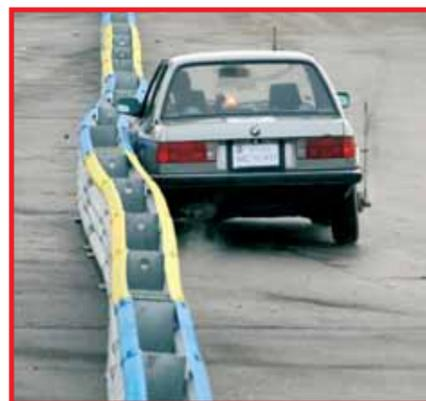
Tested in unanchored state: crash barrier systems ProTec 120 (left) and Quadro T3/W3
