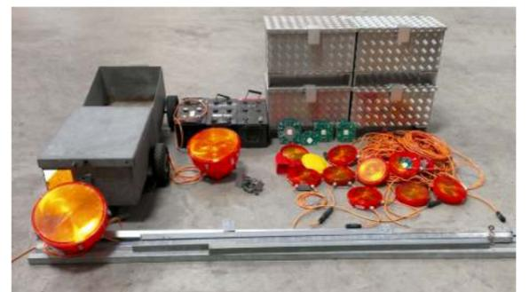
Traffic safety material found in the garden shed: LED advance warning light, temporary LED traffic control lights, control PCBs, cables, batteries etc.
