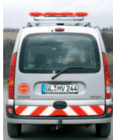
Super-flat LED illuminated arrow L15 for safeguarding the working site on a new, compact lifting and lowering device. The LED illuminated arrow with its 15 lamps is raised automatically on switching on the illuminated cross, or the "pass-right" or "pass-left" arrow.
