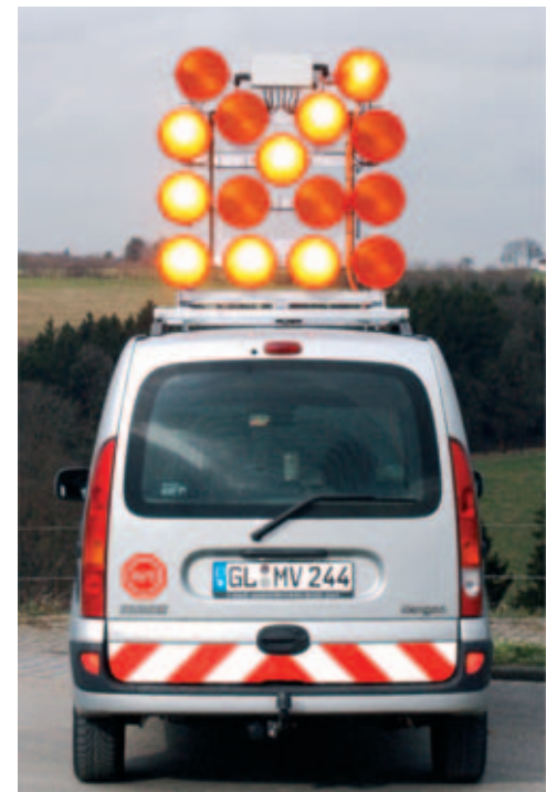
Super-flat LED illuminated arrow L15 for safeguarding the working site on a new, compact lifting and lowering device. The LED illuminated arrow with its 15 lamps is raised automatically on switching on the illuminated cross, or the "pass-right" or "pass-left" arrow.
