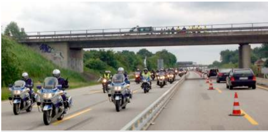
Police escort for a motorbike convoy on the A7 motorway. In the interests of safety through the roadworks, an 11 km section of the fast lane for oncoming traffic was briefly closed off with around 650 TL directing cones by AVS Hamburg at the request of the police.
