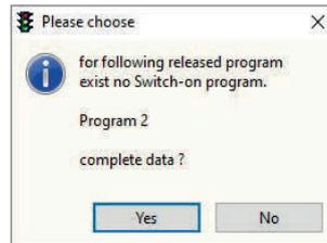
Depending on the confirmation, the editor for the switch-on programs is closed and the data are saved. **Yes** keeps the editor for the switch-on program open and you can make corrections.
