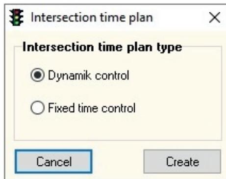
Either a fixed phase program (fixed cycle) or vehicle-actuated program (variable cycle) is created depending on the confirmation.
