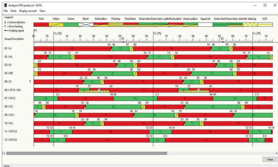
The analysis shows the signal group names for each group, the expired green phases and also the duration of the red-yellow and yellow phases, depending on the settings. At the end of each cycle, a dividing line appears with time details for the duration of the last cycle.
