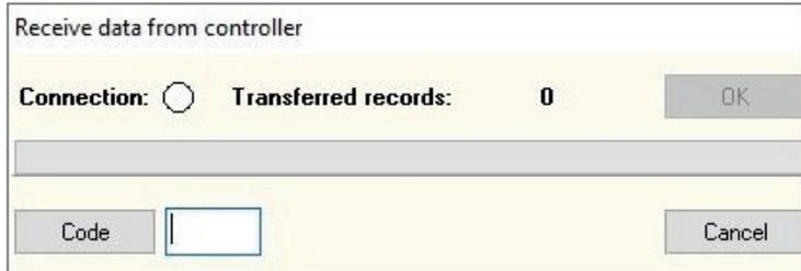
During data transfer, a progress bar shows the number of records and the status of data transfer. Depending on controller type and version, the number of transferred records can be up to 399. Press Cancel to cancel the active data transfer.
