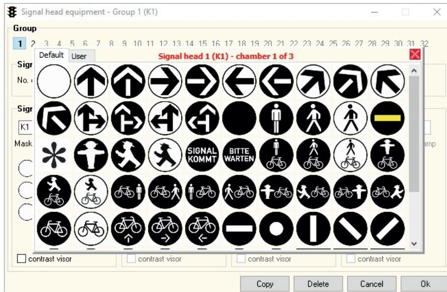
Click the left mouse button on one of the symbols to use this symbol for the corresponding signal head chamber. The selection box always shows the active signal head and the corresponding chamber for better guidance.
