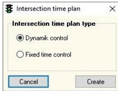
The intersection time plans are then created automatically, depending on the confirmation. On creating the intersection time plans as vehicle-actuated program, an extension point is always set one second before green end. The default time gap is 5 seconds. The minimum release time corresponds to the time entered in the signal group master data. The intersection time plan then opens automatically to check the intersection time plans.
