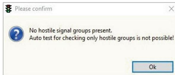
If this is confirmed, the auto test continues if other tests were selected (status, lamp monitoring). Auto test does not start if no other tests are selected.
