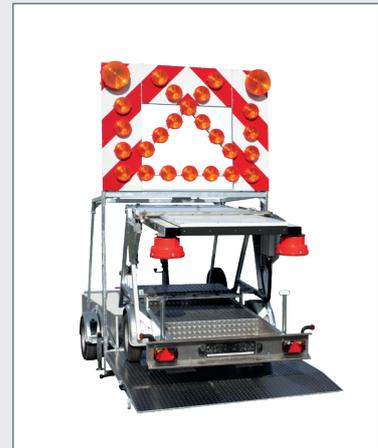
Brought quickly and efficiently to the scene with just one towing vehicle mobile warning trailer AM 4 TL carrying the mobile prewarner MV-LED.
