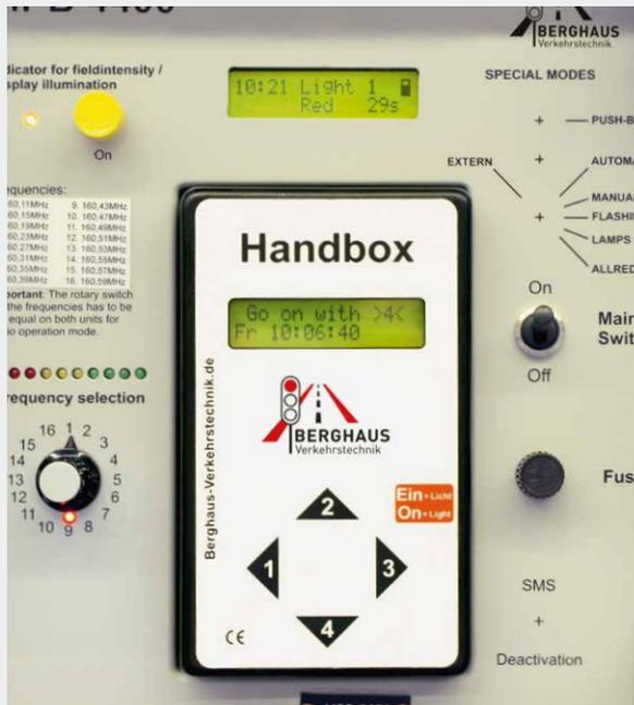
Simple handling with menu-driven handheld terminal for up to 4 signal groups. When programmed with a laptop, it is possible to control up to 12 groups and maximum 24 monitored and 24 parallel signal heads.
